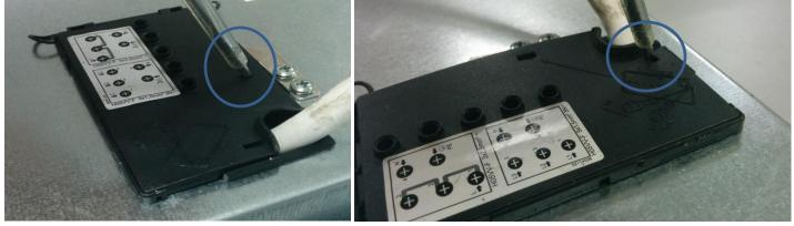
Check wiring or change according to sticker on terminal box
